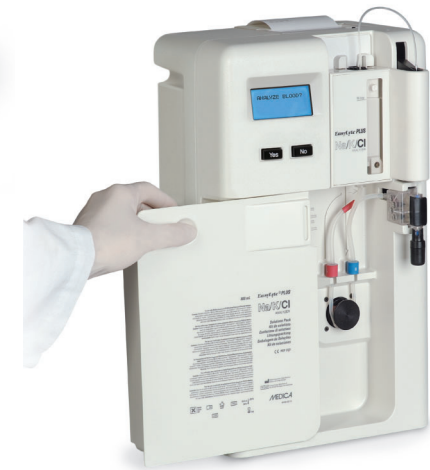
Self-contained Solutions Pack contains liquid calibrants and collects all waste, eliminates sample contact
