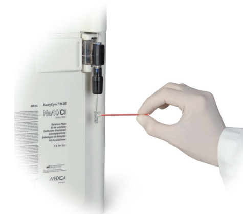
Capillary sampler is removable and disposable
