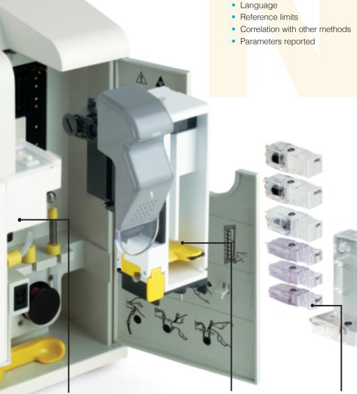
Valve Module selects calibrants and rinse solutions Sensor Module contains universal sampler with self-wiping probe for convenience and safety
