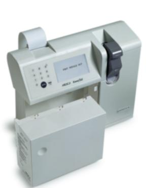
Self-contained Reagent Module contains liquid calibrants and collects all waste
